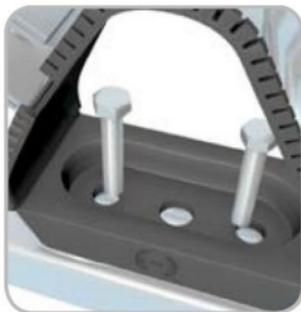
**2** Secure cleat to mounting surface using 2 x M10 or 1 x M12
